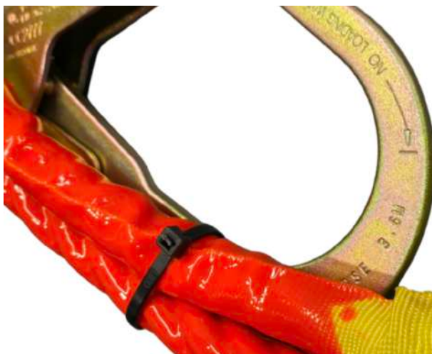
FIG 9.3. SafeGuider® attachment hook. The permanently stamped rating marking is visible on the hook body. Confirm the stamped value before each use period. The hook must be fully engaged and the self-locking mechanism closed before the crane takes the load.
