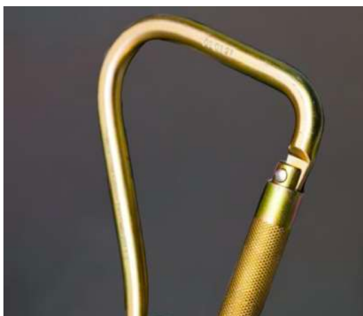
FIG 9.2. LoadGuider® rated carabiner. The knurled locking sleeve must be rotated to the locked position before lifting begins. A carabiner that does not lock positively must be removed from service.
