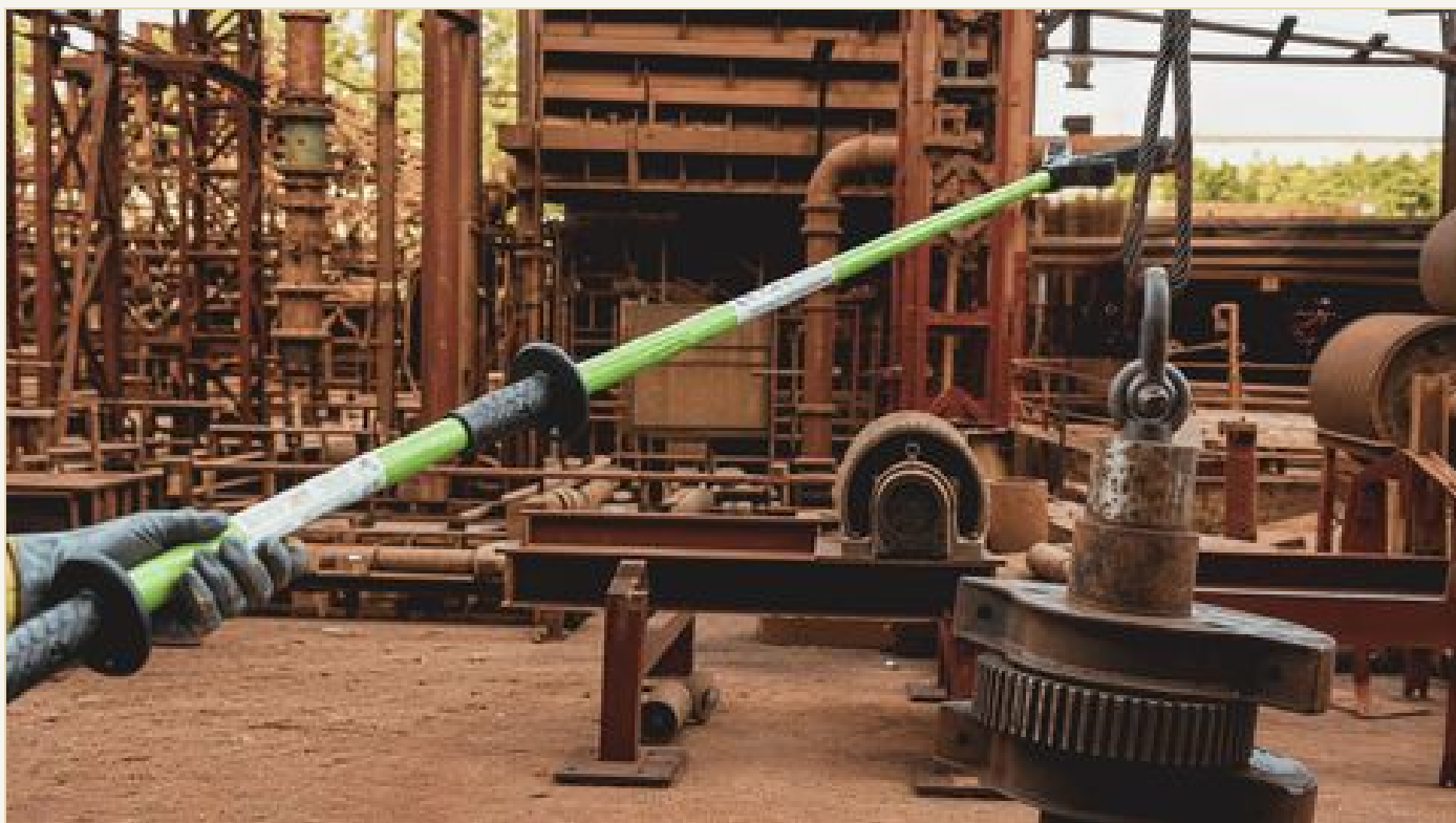
PSC LOADGUIDER® IN ACTIVE USE · HEAVY INDUSTRIAL ENVIRONMENT · WORKER MAINTAINS FULL STANDOFF DISTANCE FROM THE LOAD
