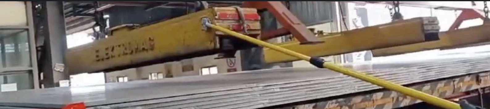
Fixed magnetic tool guiding steel plate stack — crane-assisted operation
